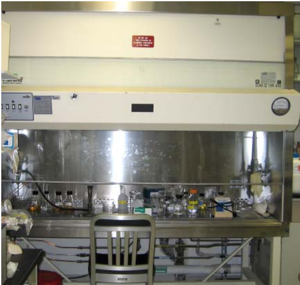
Fig. 50. A laminar hood, suitable for preparing spawn. However, clutter is not permissible.
