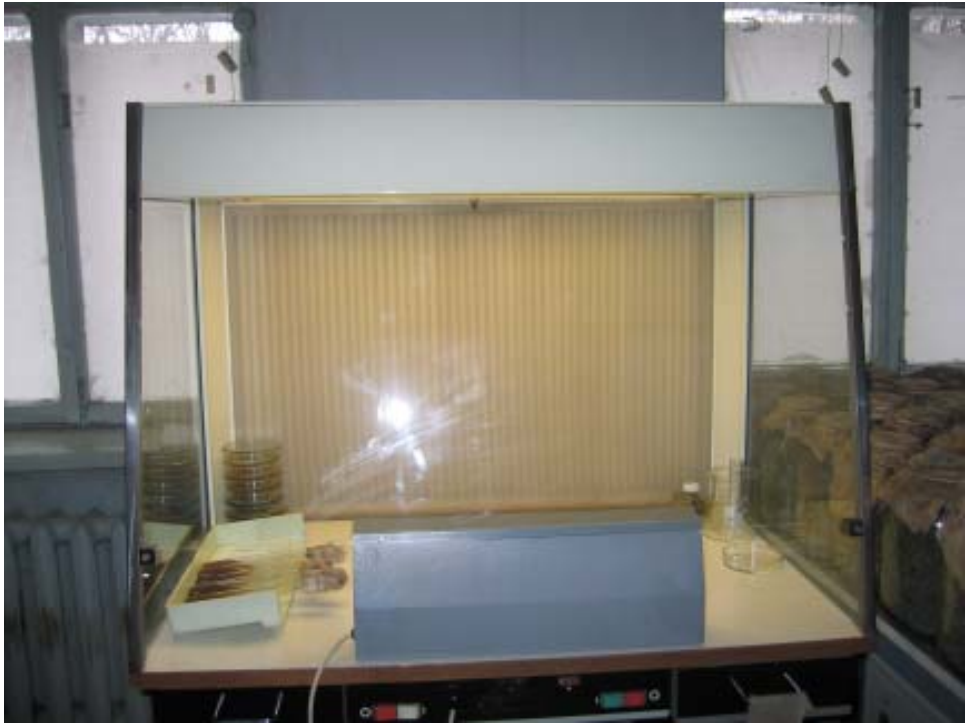
Fig. 52. A small laminar hood, suitable for work with small containers. For example starting new cultures and inoculating agar slants.
