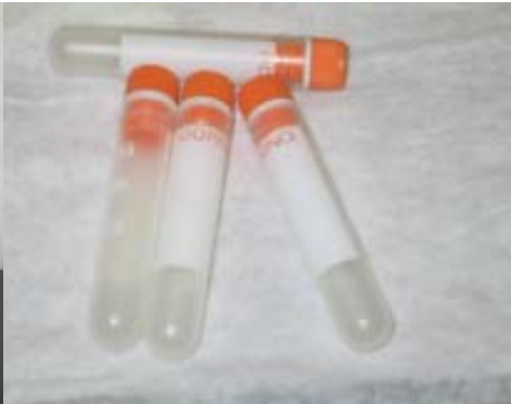
Fig. 54b. Plastic ampules also used to store mycelium in a liquid nitrogen refrigerator.
