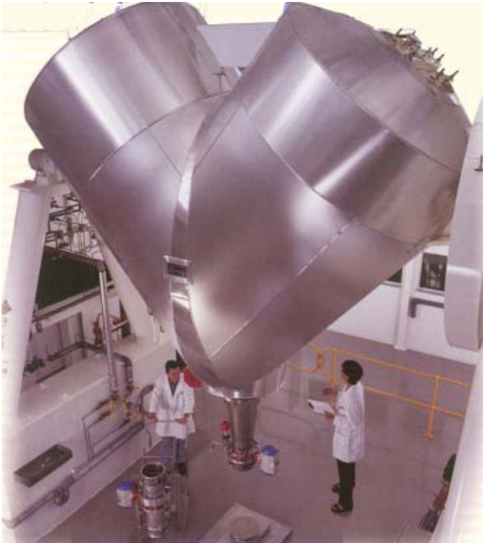
Fig. 56. A v-blendor, used by a major spawn maker to sterilize the grain for spawn. The blender rotates while high-pressure steam is put into the blender. Since the grain is kept loose, heat penetrates quickly to sterilize.
