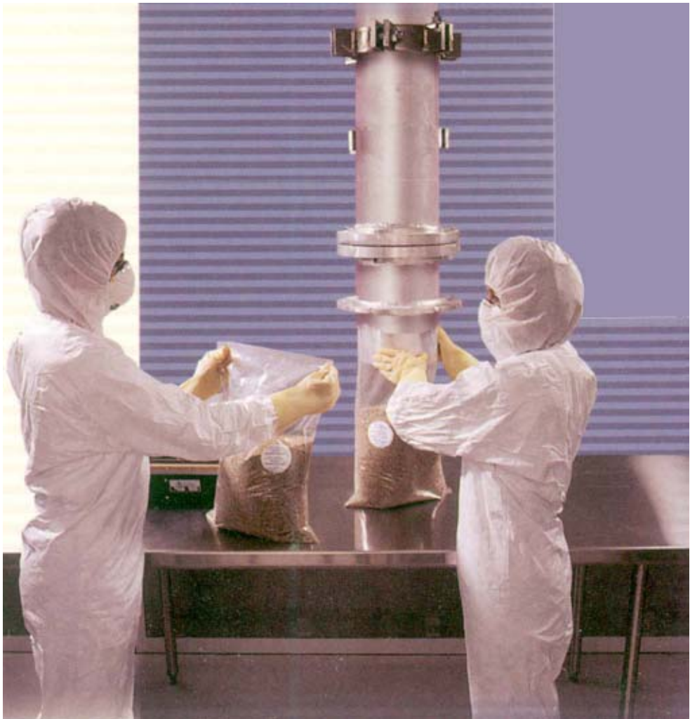
Fig. 57. Filling bags with sterile grain from the v-blender ( Fig. 56 ).
