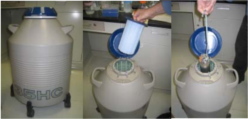
Fig. 55. A liquid nitrogen refrigerator.
