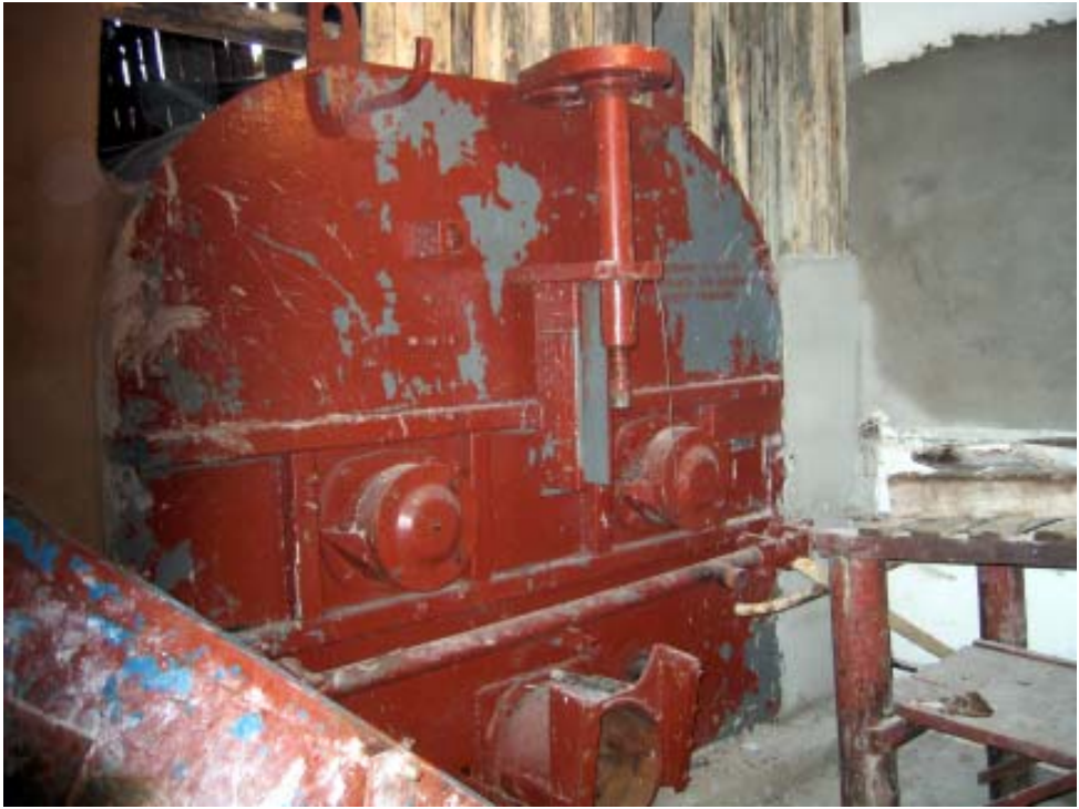
Fig. 11. End of a double shafted mixer. Note the bearings, which are at the ends of the mixing shafts and the screw conveyor at the bottom. (Belarus)
