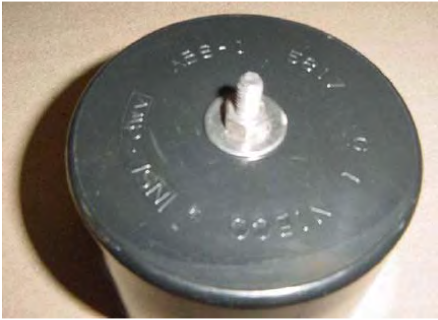
This is the Positive battery connection.
