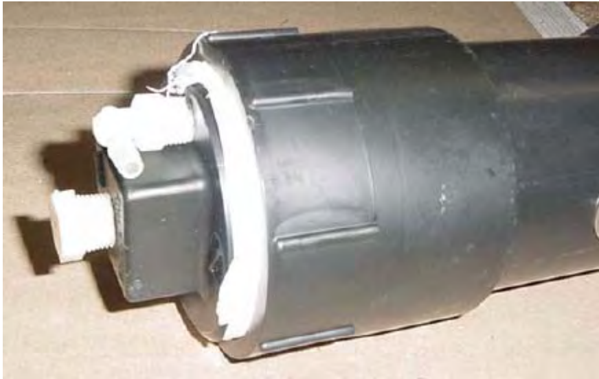
Use white "plumber's tape" on all threaded fittings.
