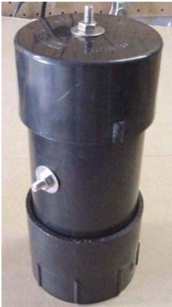
This is the finished cell shown here upside down. Assemble the unit using ABS glue.
